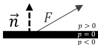
Figure 5: Computing transitions by evaluating the projection of the vector field on the normal vector
